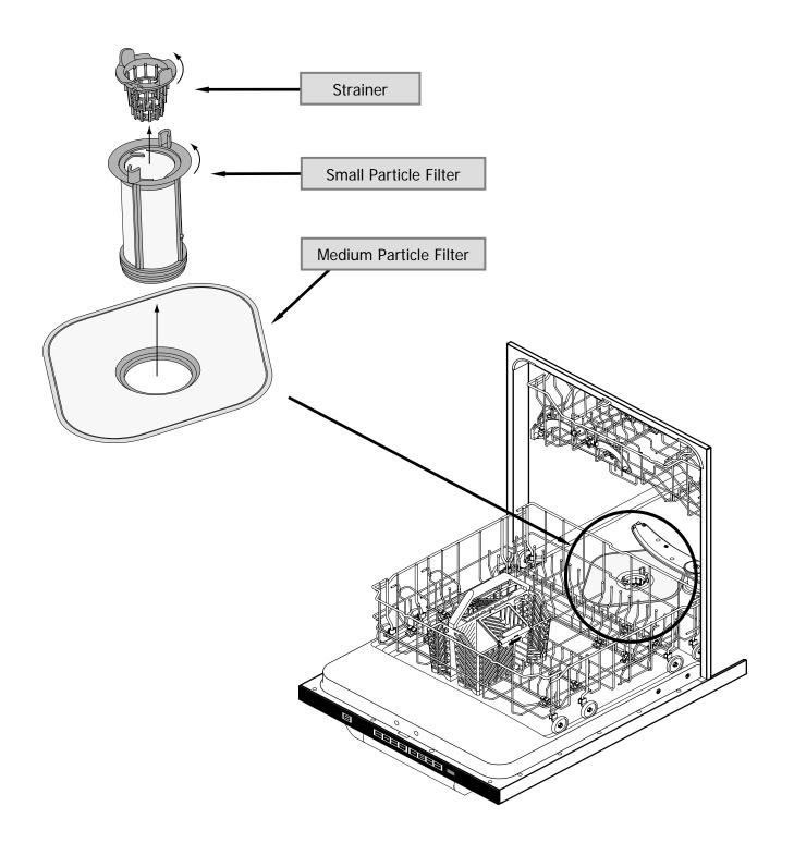
**Removing the Strainer and Filters**
